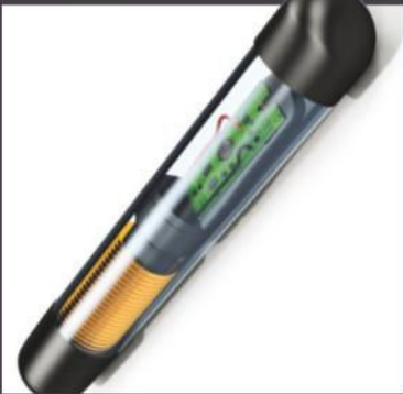
This RFID chip shows the coiled copper antenna it uses to communicate
